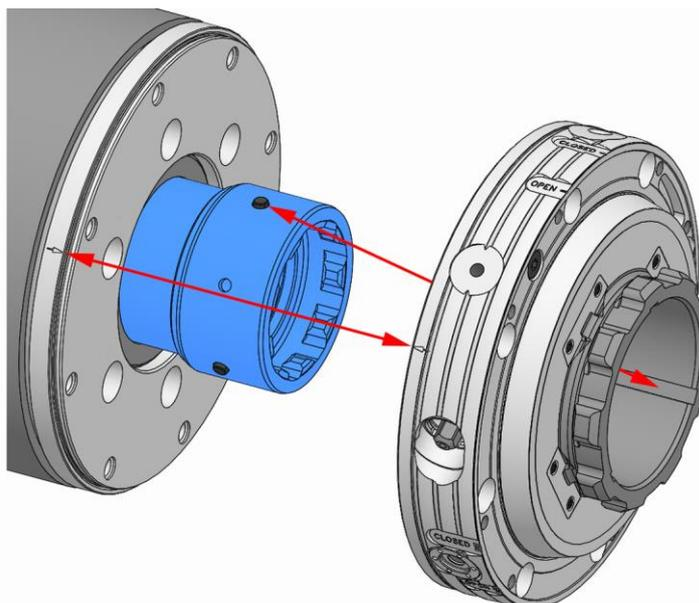
5. Remove the actuating unit from the spindle flange.
