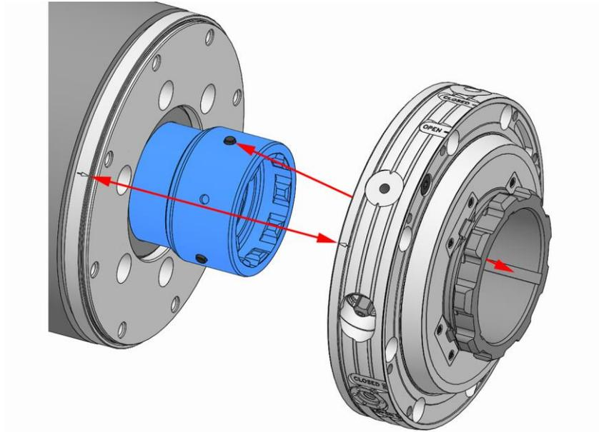
5. Fit the actuating unit on the spindle flange with the grooves in the actuating unit and the anti-twist device aligned with one another. For this, the marking on the spindle flange and the actuating unit must be aligned. For this, if necessary, twist the bayonet drawtube adapter.
