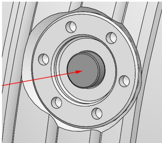
If the display pin protrudes after the locking screw has been tightened to the specified tightening torque, the quick change-over unit / quick change-over adapter has not been installed correctly. Use of the quick change-over system is prohibited if the quick change-over unit / the quick change-over adapter has not been installed correctly. The quick change-over unit / the quick change-over adapter must be installed again and the installation work must be inspected.
