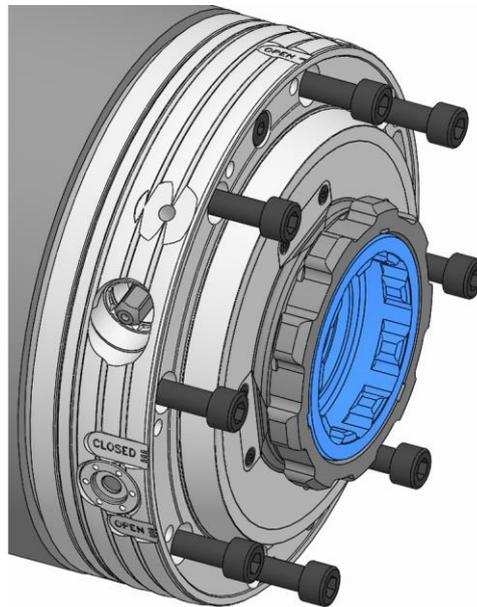
6. Screw the fixings crews into the actuating unit and tighten them gently.
