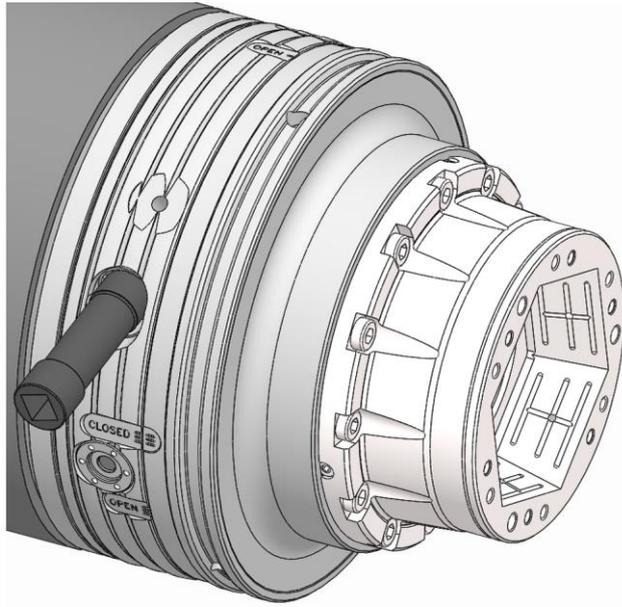
6. Using the actuating key, turn the locking screw counter-clockwise until it reaches the stop without exerting any force.
