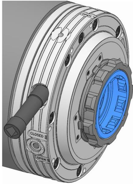
7. Using the actuating key, turn the locking screw counter-clockwise until it reaches the stop without exerting any force.
