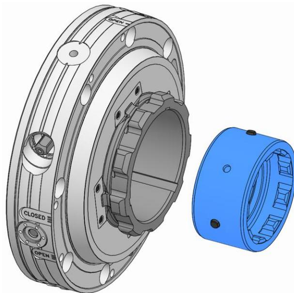
3. Remove the bayonet drawtube adapter from the actuating unit.
