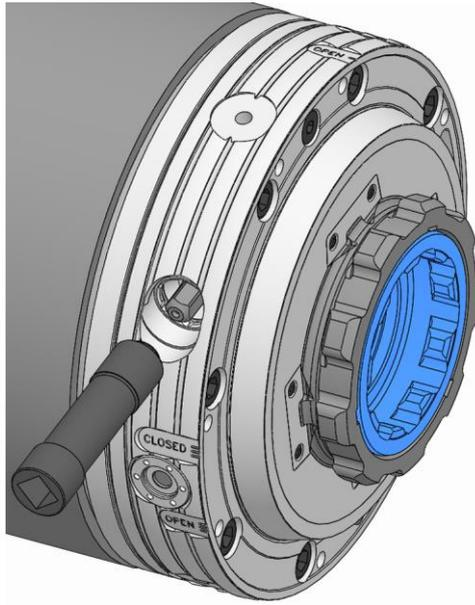
10. Fit the actuating key to the locking screw and hold it firmly.
