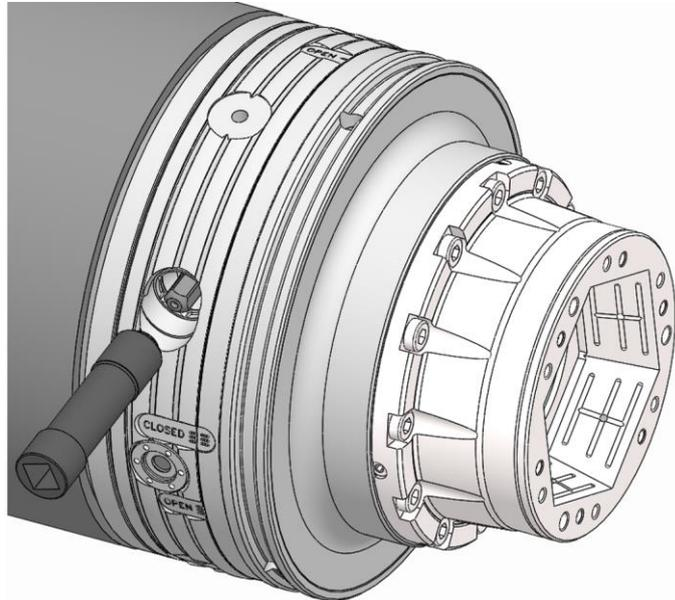
5. Fit the actuating key to the locking screw and hold it firmly.
