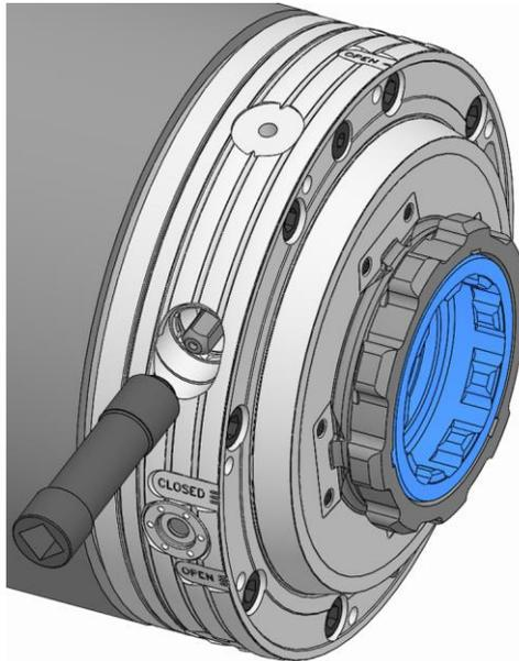
6. Fit the actuating key to the locking screw and hold it firmly.
