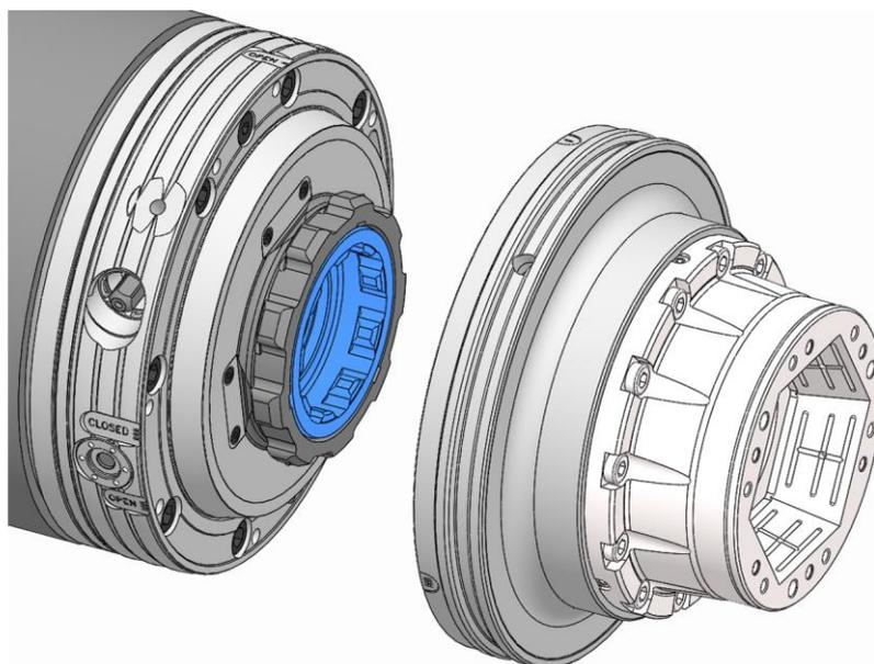
9. Fit the quick change-over unit to the machine adapter so that the mark on the quick change-over unit is aligned with the »OPEN« mark on the machine adapter.
