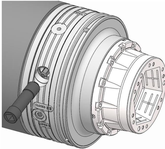
7. Remove the actuating key from the locking screw and remove it from the working area of the machine.
