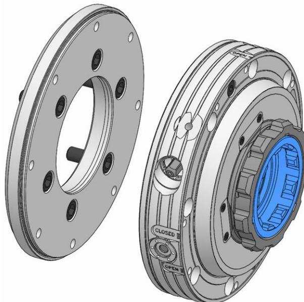
2. Remove the actuating unit from the spindle flange.
