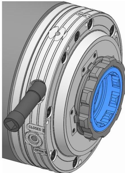
11. Turn the locking screw with the help of the actuating key until the bayonet of the actuating unit is not in a limit position.
