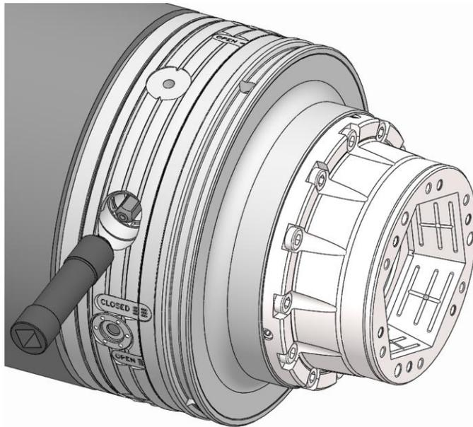
14. Remove the actuating key from the locking screw and remove it from the working area of the machine.
