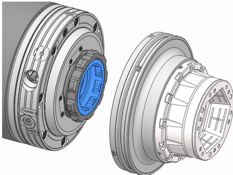
9. Take down the quick change-over unit from the machine adapter.
