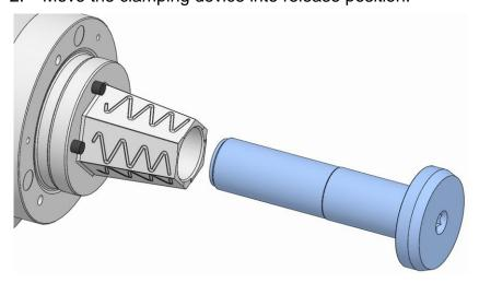
3. Unfasten and remove the tension bolt.
