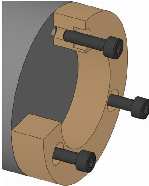
1. Unfasten and remove the fixing screws on the changing part.
