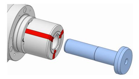
Unfasten and remove the tension bolt.
