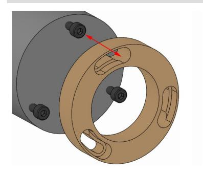
Place the changing part on the product so that the screw head on the changing part fixing screw fits through the bayonet opening.
