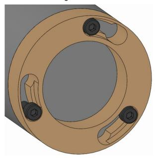
2. Turn the changing part until the screw head on the changing part fixing screw fits through the bayonet opening.
