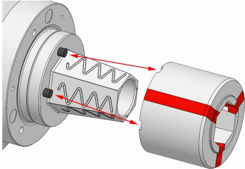
4. Fit the segmented clamping bushing to the product. For this, the grooves in the segmented clamping bushing must engage in the ejector pins.
