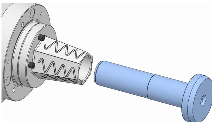
3. Unfasten and remove the tension bolt.
