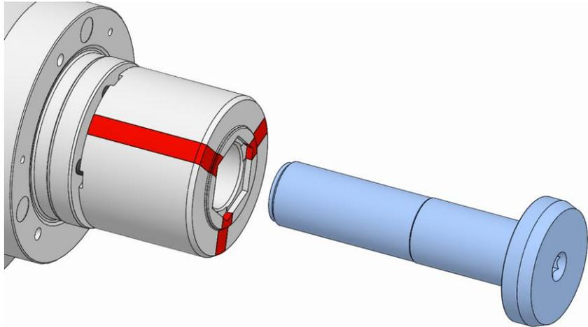
3. Unfasten and remove the tension bolt.
