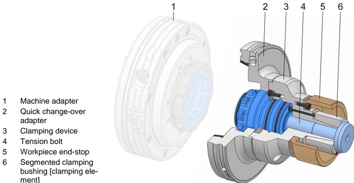
The machine adapter is secured to the machine spindle.
