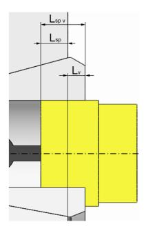
Without exception, never go below the total clamping length  $L_{sp\ v}$  of the workpiece, which measures at least 8 mm.
