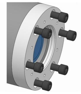
4. Screw in the changing part fixing screws on the spindle flange and tighten to the specified tightening torque [see »Screw tightening torques« chapter].
