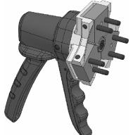
The pins on the changing fixture are installed in the changing bores in the clamping head. The changing fixture is actuated by manual force. Depending on size, the changing fixture may be designed for single-handed or for twohanded actuation. The clamping head is clamped firmly in the changing fixture and can be installed in the mounted clamping device with the help of the changing fixture.
