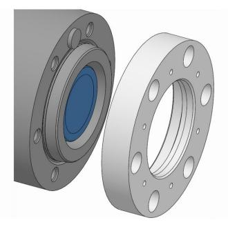
4. Take down the spindle flange from the machine spindle. **10.5.3Removal of the drawtube adapter**
