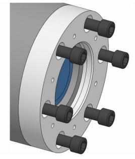
3. Unfasten and remove the fixing screws on the spindle flange.
