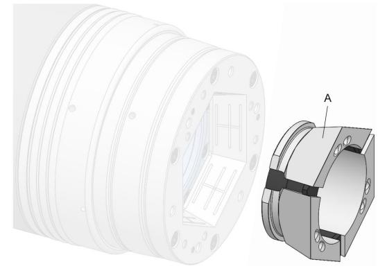
A Clamping head [clamping element]
