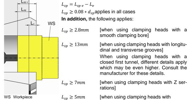
If HAINBUCH uses a different and shorter clamping length in this clamping situation drawing, this will have been checked against the specific parameters for this type of application and found to be sufficient.
