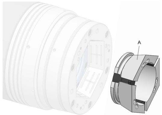
A Clamping head [clamping element]
