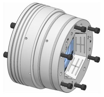
2. Unfasten and remove the fixing screws on the functional unit.
