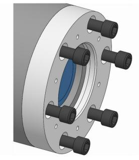
4. Screw in the spindle flange fixing screws and tighten them gently.
