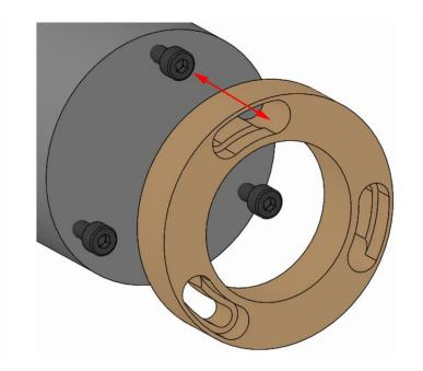
3. Take the changing part off the product. **10.3.4Removal of the central variant with axial screw connection**
