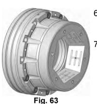
4. Remount the clamping devices. Re-insert the clamping unit in the spindle flange.
