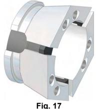
The clamping heads are used to accommodate the work piece that will be machined. They consists of hard steel and rubber segments that are connected via a vulcanizing process.
