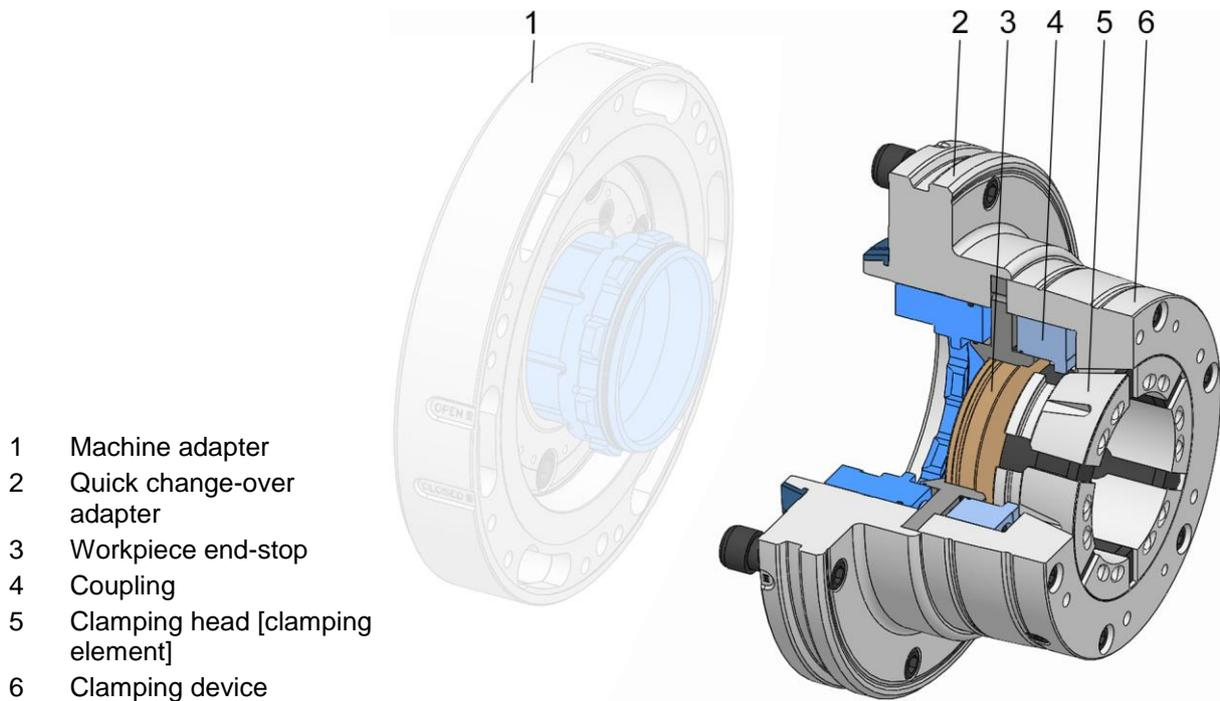
The clamping device can be used as a through-chuck for machining bar stock and also as an end-stop chuck.
