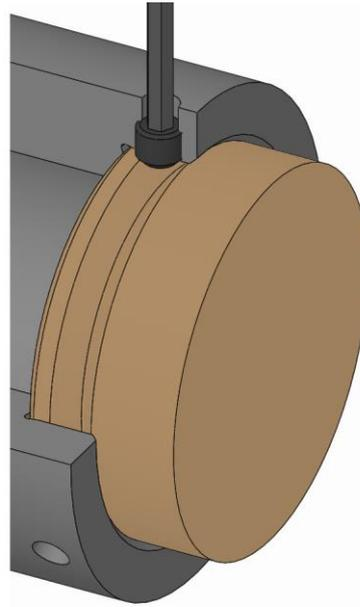
2. Screw in the clamping screws on the changing part and tighten to the specified tightening torque [see Nomenclature].
