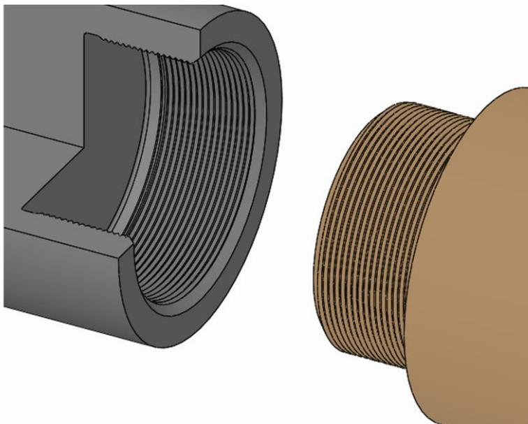
1. Screw the changing part into the product using its thread, and tighten it down.
