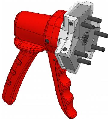
The pins on the changing fixture are installed in the changing bores in the clamping head. The changing fixture is actuated by manual force. Depending on size, the changing fixture may be designed for single-handed or for two-handed actuation. The clamping head is clamped firmly in the changing fixture and can be installed in the mounted clamping device with the help of the changing fixture.
