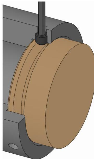
1. Unscrew the clamping screws from the changing part until the changing part can be lifted out.
