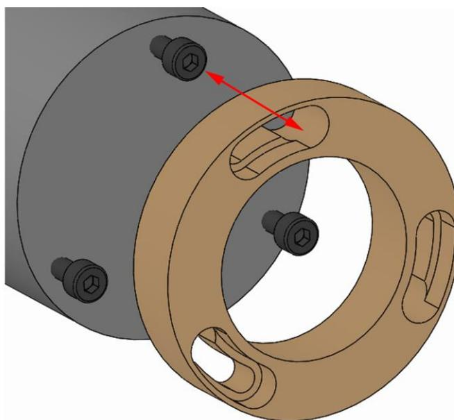
1. Place the changing part on the product so that the screw head on the changing part fixing screw fits through the bayonet opening.
