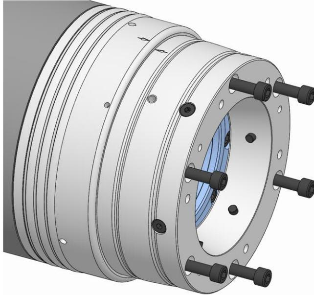
4. Unfasten and remove the fixing screws on the functional unit.
