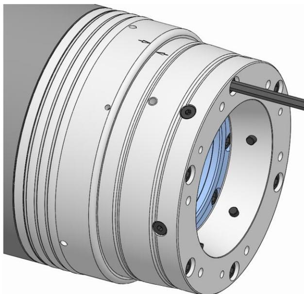
11. Tighten the fixing screws on the functional unit to the specified tightening torque [see »Screw tightening torques« chapter].
