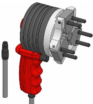
The pins on the changing fixture are installed in the changing bores in the clamping head. The changing fixture is actuated pneumatically. Depending on size, the changing fixture may be designed for single-handed or for two-handed actuation. The clamping head is clamped firmly in the changing fixture and can be installed in the mounted clamping device with the help of the changing fixture.
