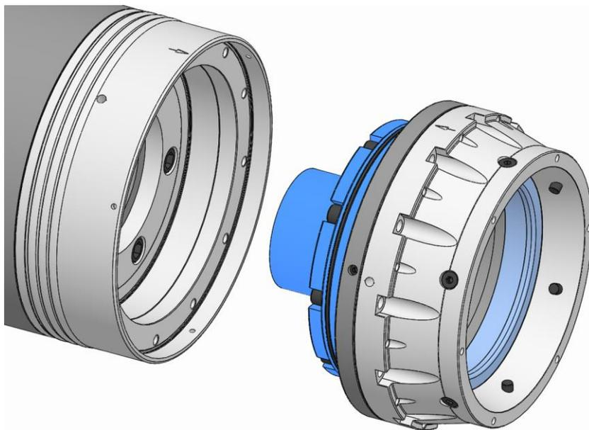
9. Take down the functional unit from the spindle flange.
