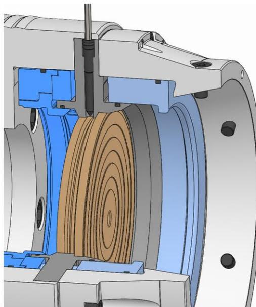
1. Unscrew the clamping screws from the base end-stop until the base end-stop can be lifted out.
