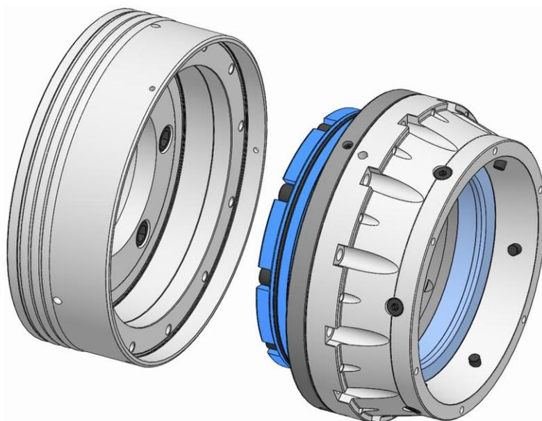
5. Take down the functional unit from the spindle flange.
