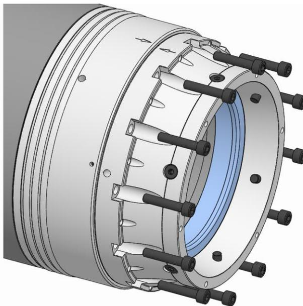
9. Screw in the fixing screws on the functional unit and tighten to the specified tightening torque [see »Screw tightening torques« chapter].
