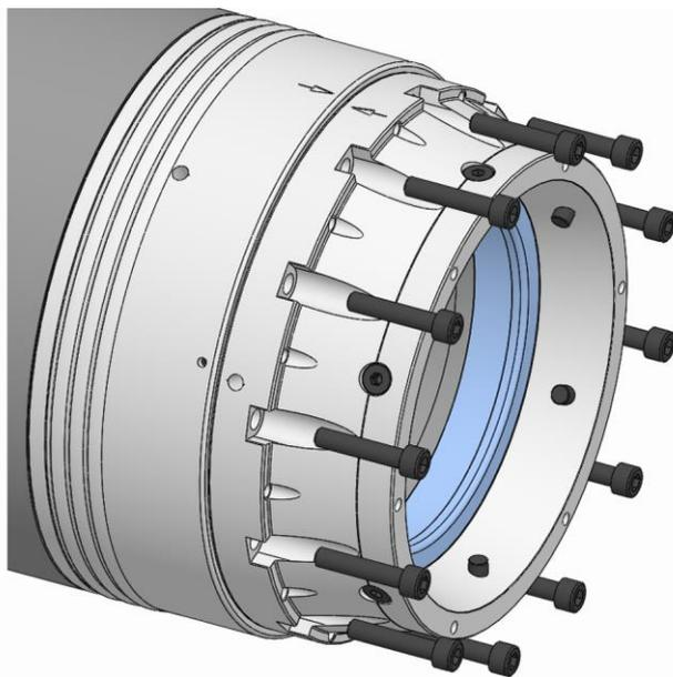
9. Screw in the fixing screws on the functional unit and tighten them gently.
