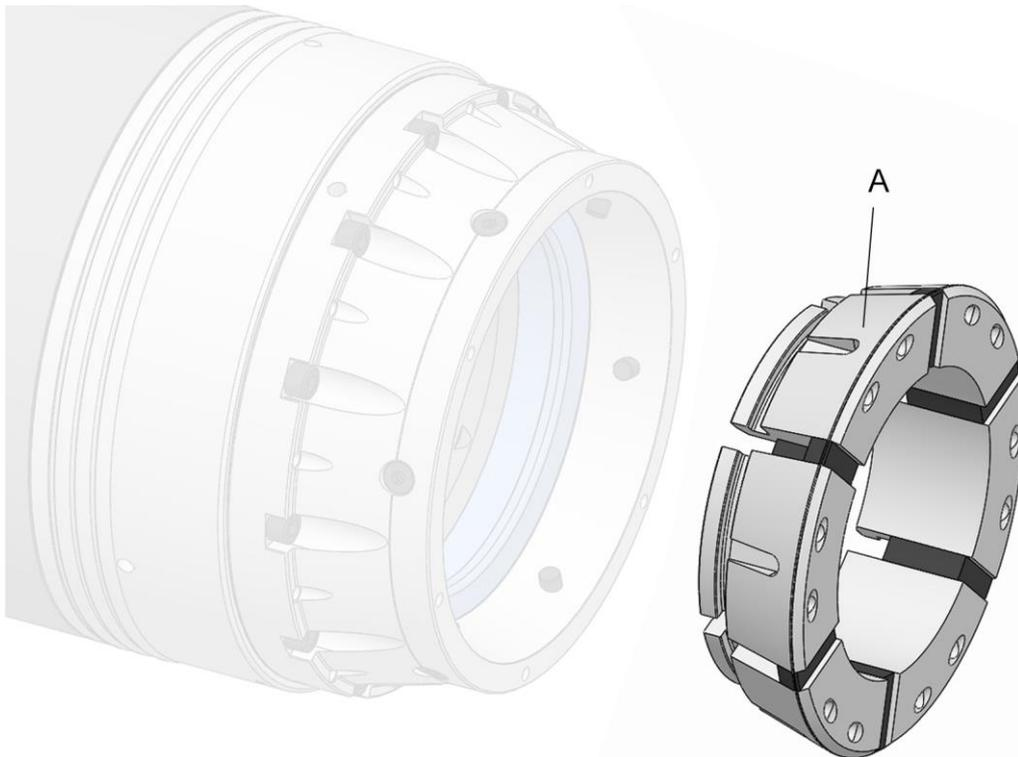
A Clamping head [clamping element]
