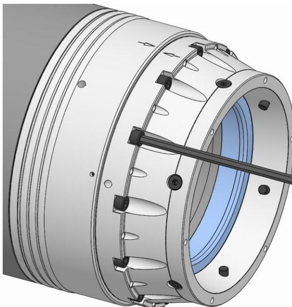
13. Tighten the fixing screws on the functional unit to the specified tightening torque [see »Screw tightening torques« chapter].
