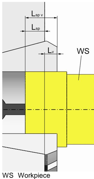
The clamping length is calculated as follows:
