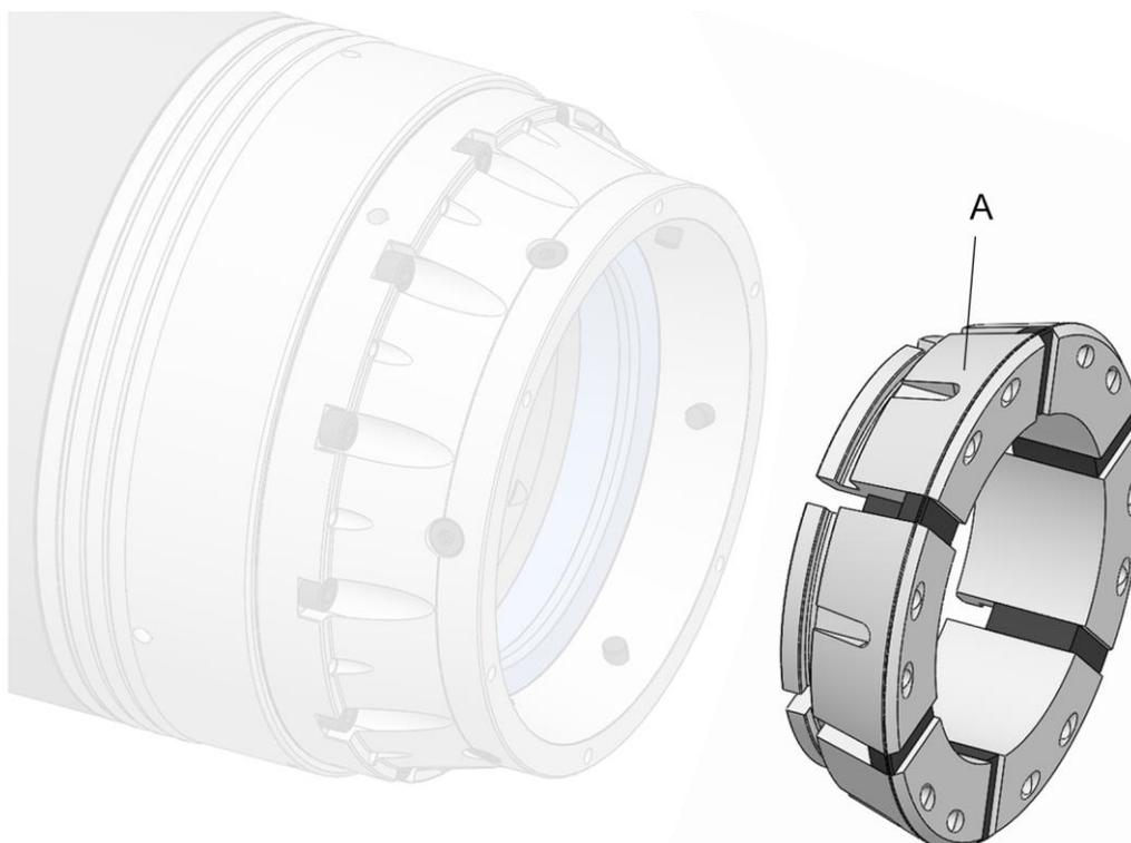
A Clamping head [clamping element]
