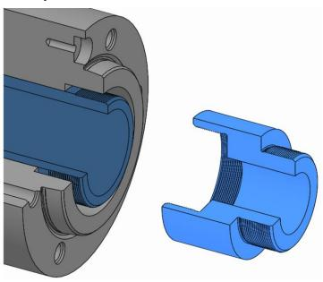
If the drawtube adapter was mounted on the machine drawtube, use its thread to unscrew and remove it from the machine drawtube.
