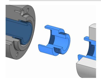
1. Screw the drawtube adapter into the functional unit using its thread or screw it to the machine drawtube and tighten it down.
