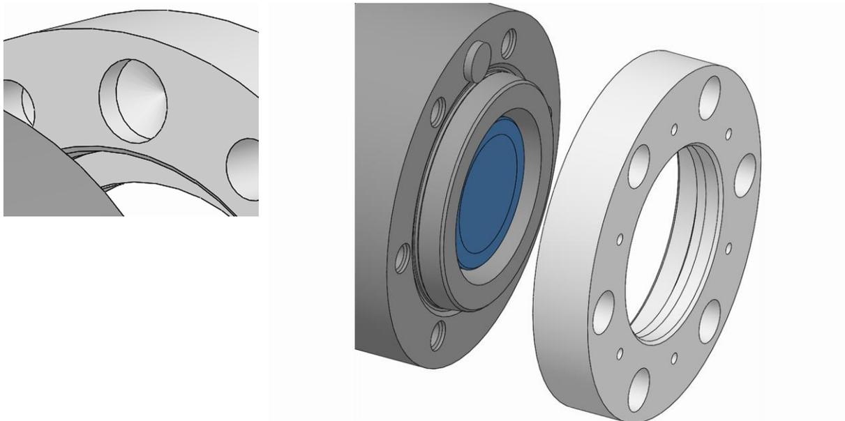
4. Take down the spindle flange from the machine spindle.
