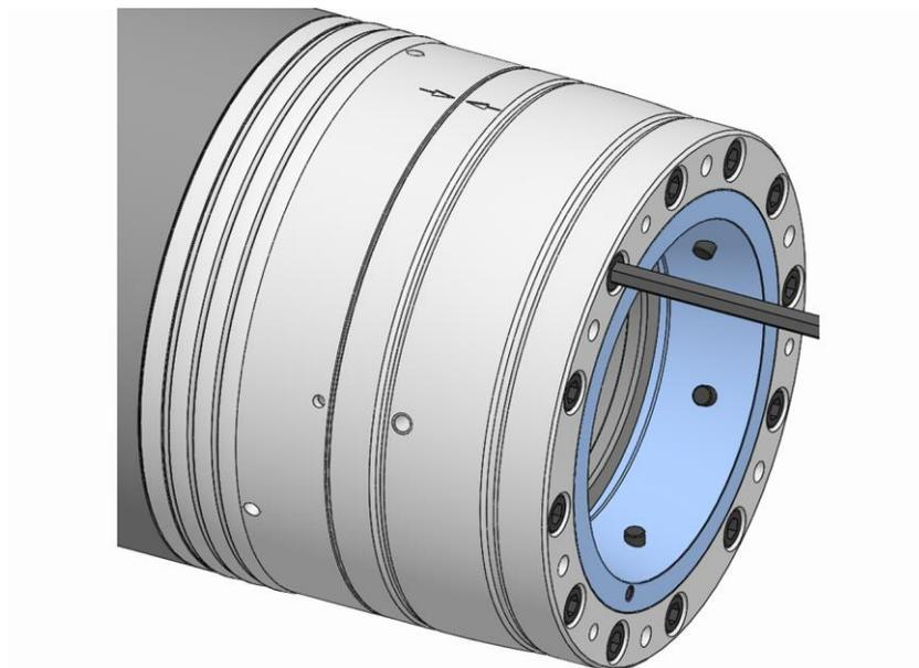
11. Tighten the fixing screws on the functional unit to the specified tightening torque [see »Screw tightening torques« chapter].
