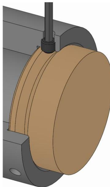
2. Screw in the clamping screws on the changing part and tighten to the specified tightening torque [see Nomenclature].
