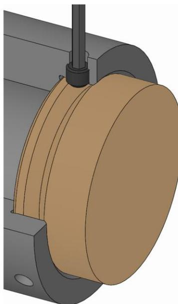
1. Unscrew the clamping screws from the changing part until the changing part can be lifted out.
