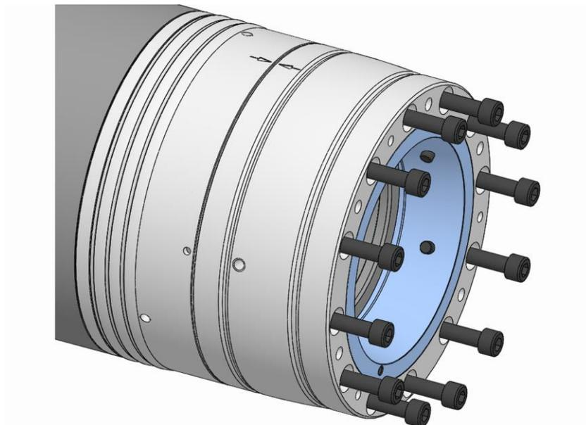
7. Screw in the fixing screws on the functional unit and tighten them gently.
