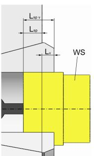
The clamping length is calculated as follows:
