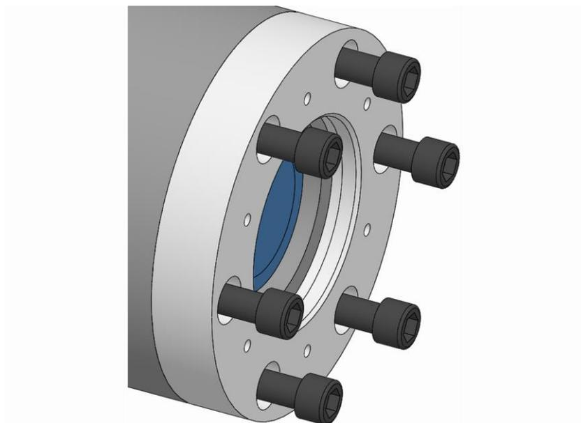
4. Screw in the changing part fixing screws on the spindle flange and tighten to the specified tightening torque [see »Screw tightening torques« chapter].
