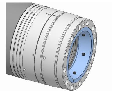
Turn back the functional unit until the balancing marks on the spindle flange are aligned with those on the functional unit.
