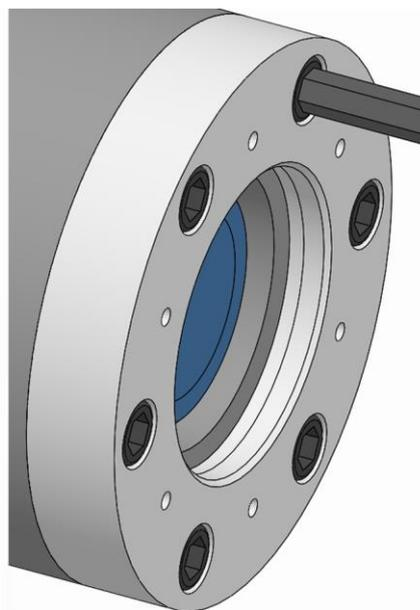
8. Screw in the drift body fixing screws on the spindle flange and tighten to the specified tightening torque [see »Screw tightening torques« chapter].
