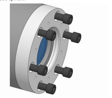
3. Unfasten and remove the fixing screws on the spindle flange.
