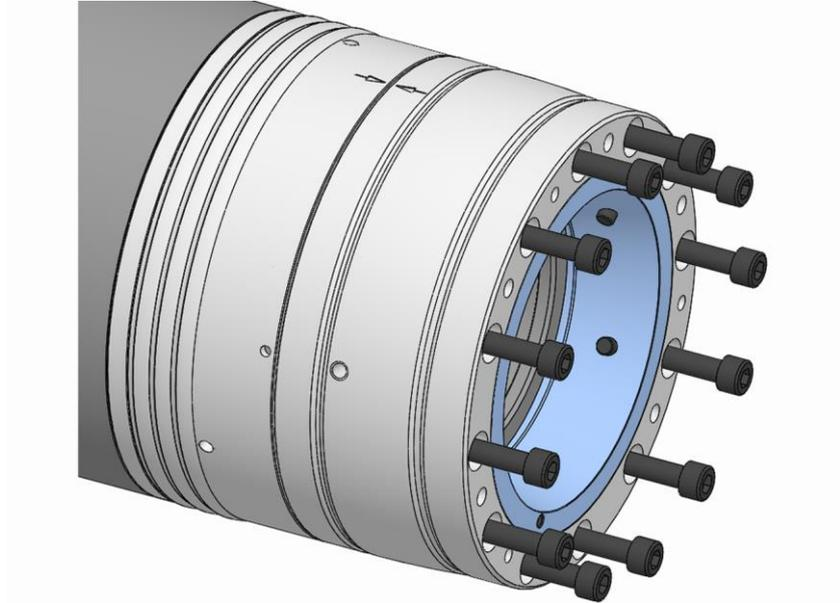
4. Unfasten and remove the fixing screws on the functional unit.
