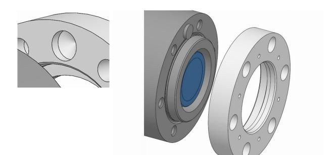
Take down the spindle flange from the machine spindle.
