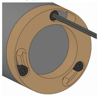
Screw in the changing part fixing screws and tighten to the specified tightening torque [see »Screw tightening torques« chapter]. 3.
