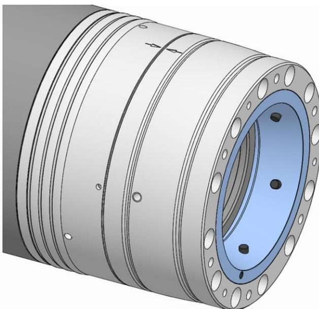
5. Turn back the functional unit until the balancing marks on the spindle flange are aligned with those on the functional unit.
