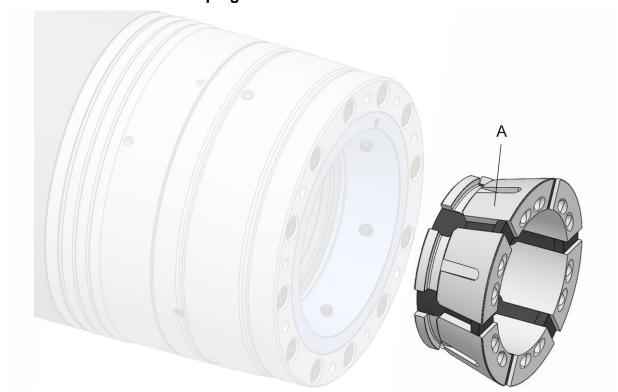
A Clamping head [clamping element]
