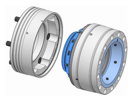
3. Take down the functional unit from the spindle flange.
