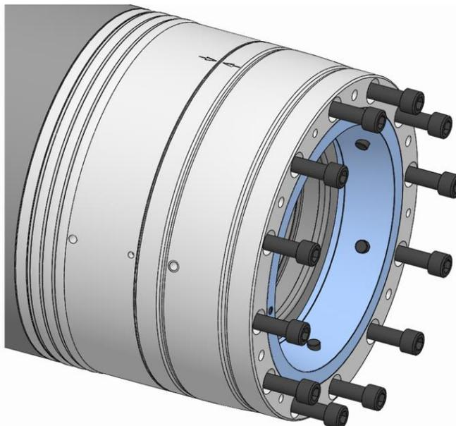
9. Screw in the fixing screws on the functional unit and tighten to the specified tightening torque [see »Screw tightening torques« chapter].
