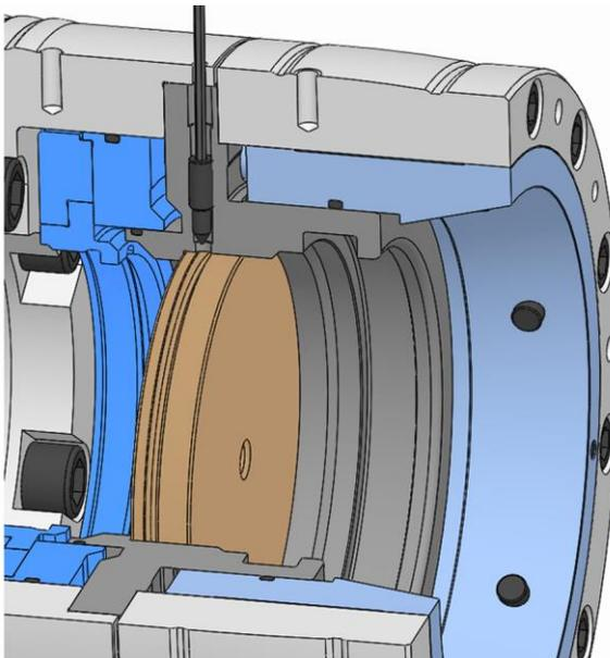
1. Unscrew the clamping screws from the base end-stop until the base end-stop can be lifted out.
