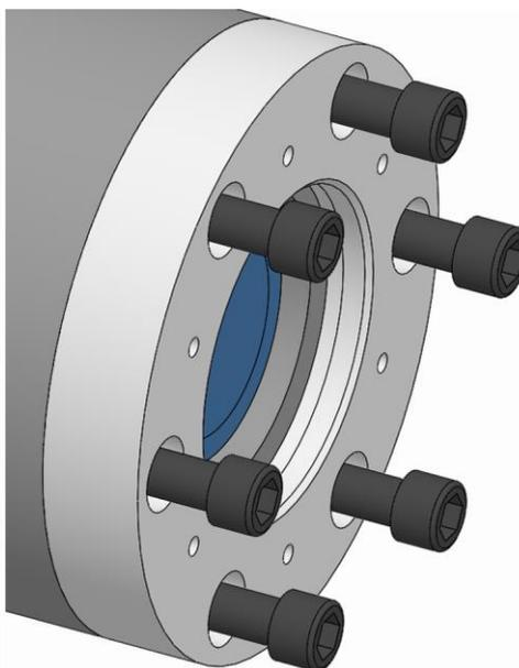
4. Screw in the spindle flange fixing screws and tighten them gently.
