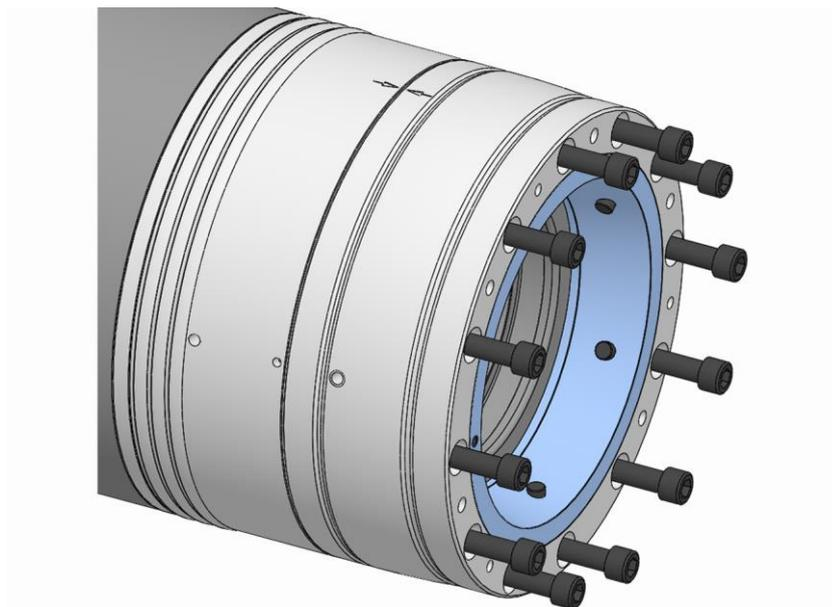
9. Screw in the fixing screws on the functional unit and tighten them gently.
