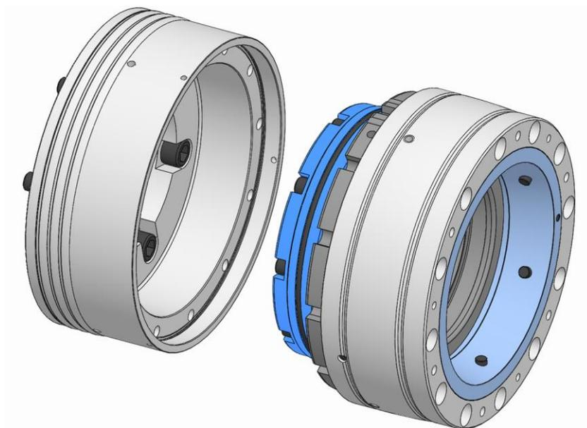
5. Take down the functional unit from the spindle flange.
