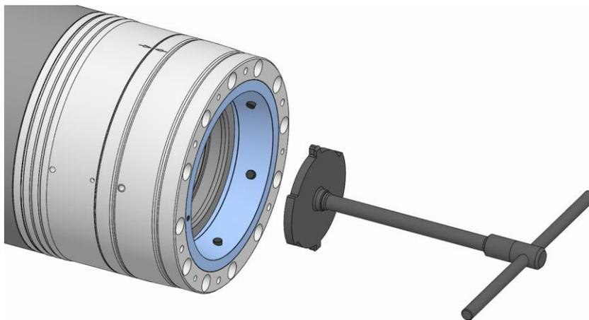
5. Install the mounting aid in the functional unit to enable the mounting aid to engage in the grooves of the drawtube adapter in the functional unit.
