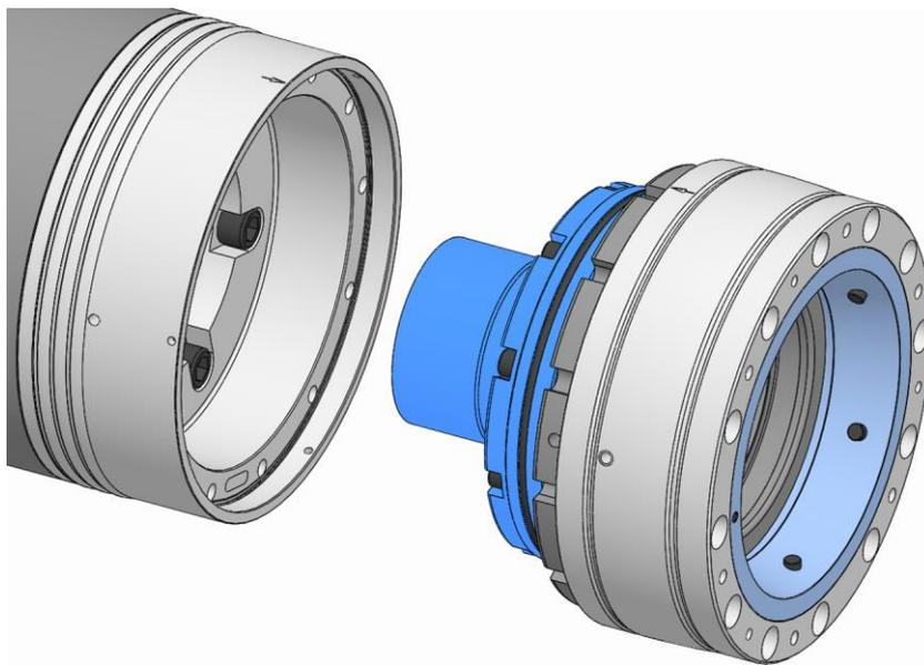
9. Take down the functional unit from the spindle flange.
