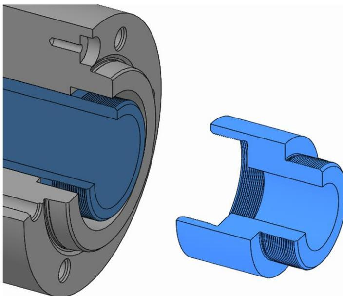
1. If the drawtube adapter was mounted on the machine drawtube, use its thread to unscrew and remove it from the machine drawtube.
