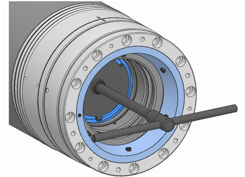
7. Using the mounting aid, unscrew and remove the draw-tube adapter on the functional unit from the machine drawtube.
