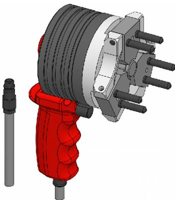
The pins on the changing fixture are installed in the changing bores in the clamping head. The changing fixture is actuated pneumatically. Depending on size, the changing fixture may be designed for single-handed or for two-handed actuation. The clamping head is clamped firmly in the changing fixture and can be installed in the mounted clamping device with the help of the changing fixture.
