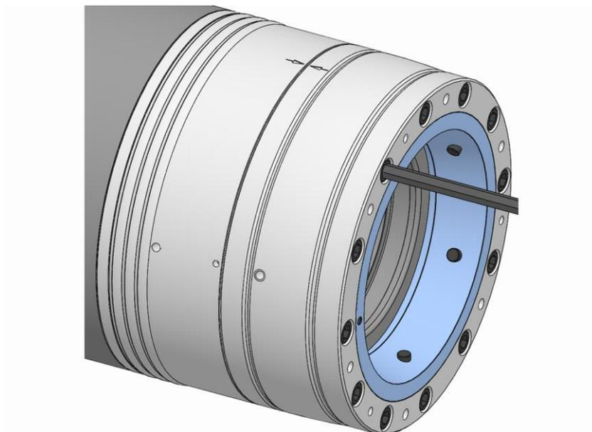
13. Tighten the fixing screws on the functional unit to the specified tightening torque [see »Screw tightening torques« chapter].
