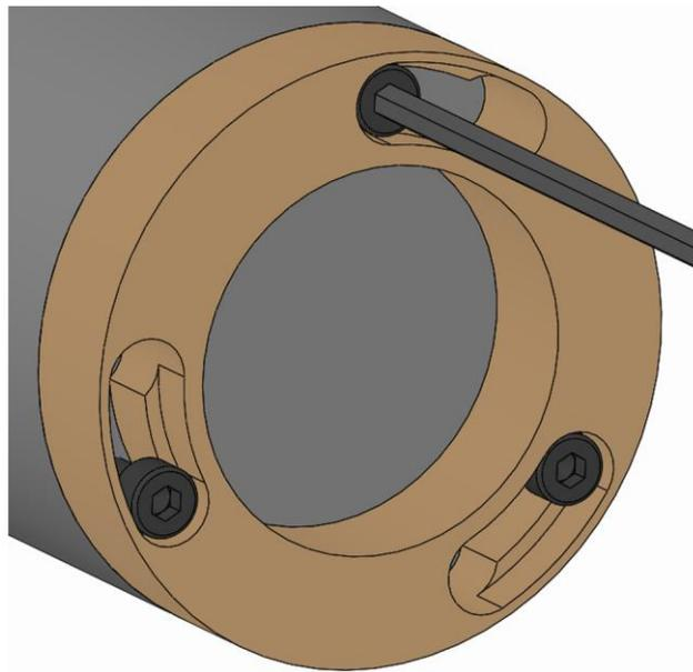
3. Screw in the changing part fixing screws and tighten to the specified tightening torque [see »Screw tightening torques« chapter].
