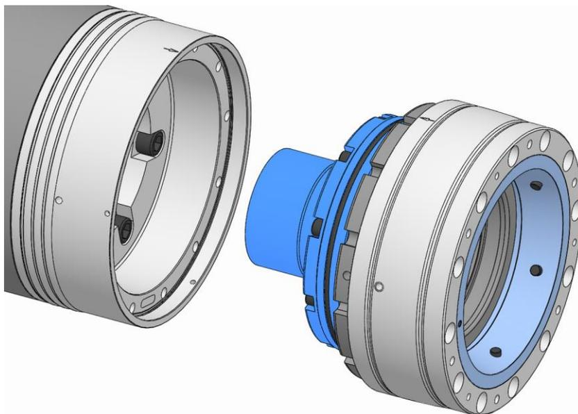
4. Fit the functional unit on the spindle flange until the balancing marks on the spindle flange are aligned with those on the functional unit.
