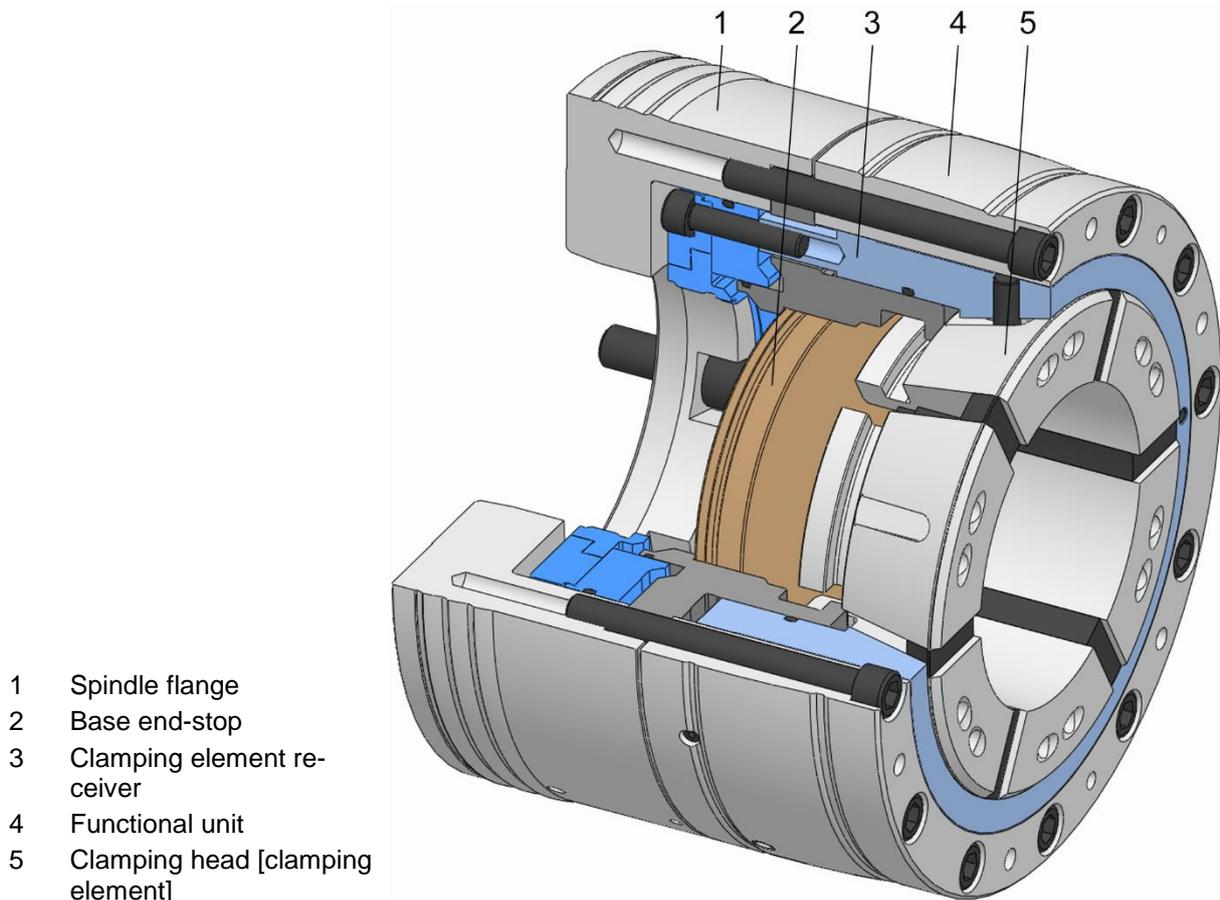
The clamping device can be used as a through-chuck for machining bar stock and also as an end-stop chuck.
