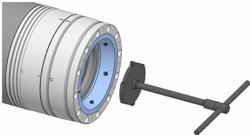
6. Install the mounting aid in the functional unit to enable the mounting aid to engage in the grooves of the drawtube adapter in the functional unit.
