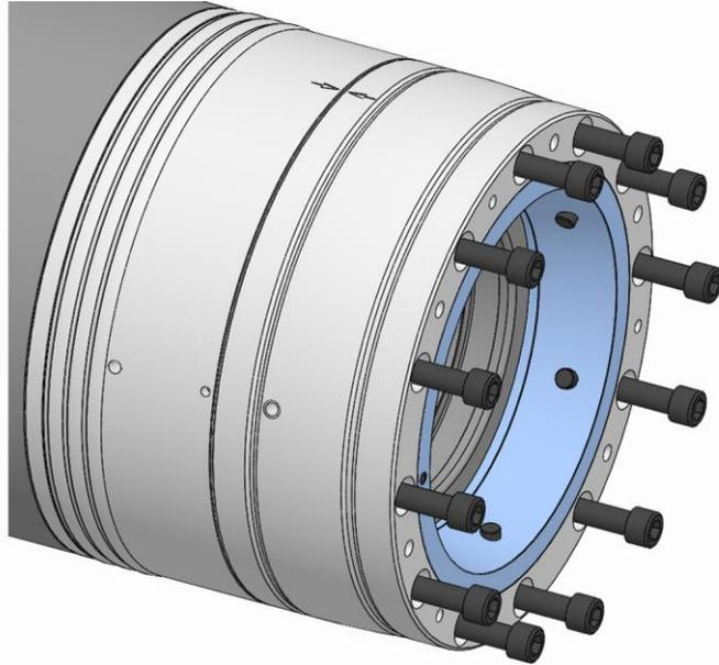
4. Unfasten and remove the fixing screws on the functional unit.
