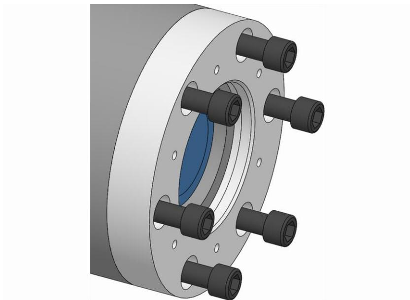
3. Unfasten and remove the fixing screws on the spindle flange.
