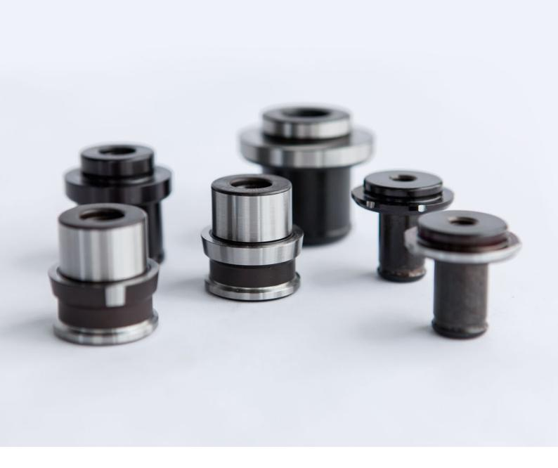
The clamping bolts are an important component of the DockLock system; they create the connection between the clamping module and the changing part. They are universal and can be inserted in the pallet, the clamping device or directly in the workpiece. Centering clamping bolts feature a high-precision collar for alignment in the clamping position of the clamping module. That ensures repeatability of  $\leq$  0.005 mm.
