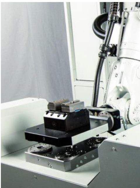
Automated change-over with the Docklock AC zero-point clamping system.
