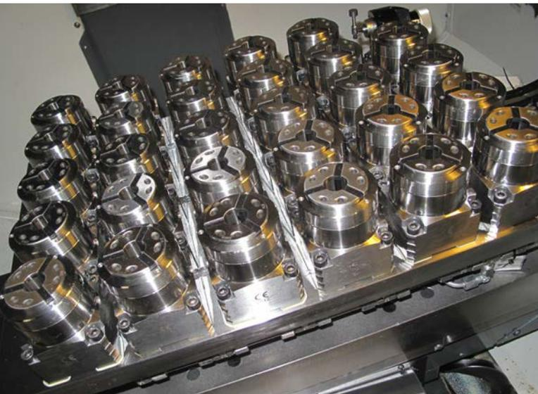
**2** Optimally utilized: Precisely 30 size-32 HYDROKs, plus traverse distances, fit on the machine table of the Haas machining center. The base plate remains stationary in the machine.
