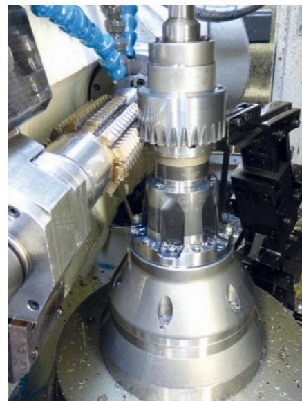
The Mando G211 mandrel on the Richardson is perfect for hobbing.
