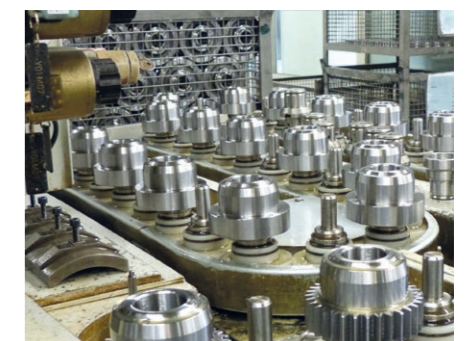
The automatic loading system with the gears on the Gleason Pfauter machine.
