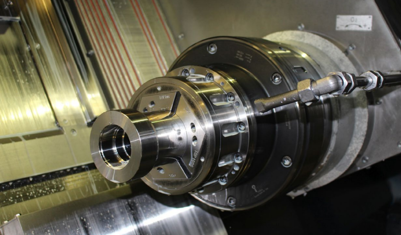
The sub spindle of the lathe is also equipped with the Centrotex adapters.
