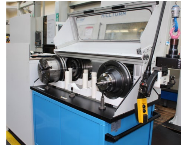
The clamping device waits to be exchanged. The placement cart is an in-house construction from Arburg.
