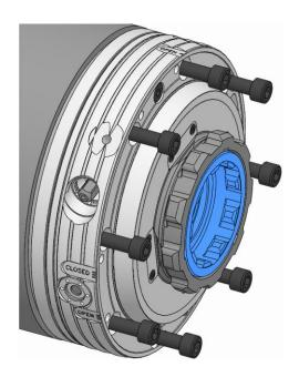
4. Unfasten and remove the retaining screws on the actuating unit.
