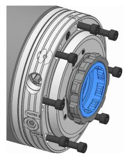
6. Screw the fixings crews into the actuating unit and tighten them gently.
