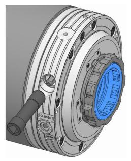
6. Fit the actuating key to the locking screw and hold it firmly.
