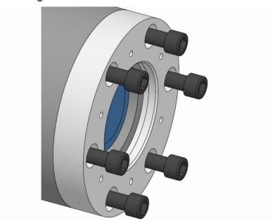
4. Screw in the spindle flange fixing screws and tighten them gently.
