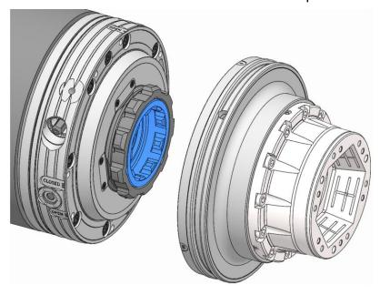
9. Take down the quick change-over unit from the machine adapter.
