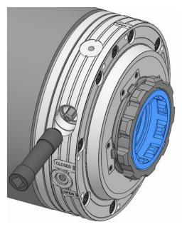
8. Remove the actuating key from the locking screw and remove it from the working area of the machine.
