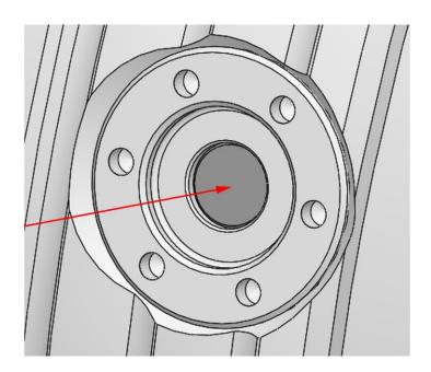
If the display pin is recessed or maximally flush after tightening the locking screw to the specified tightening torque, the quick change-over unit / quick change-over adapter has been correctly installed.
