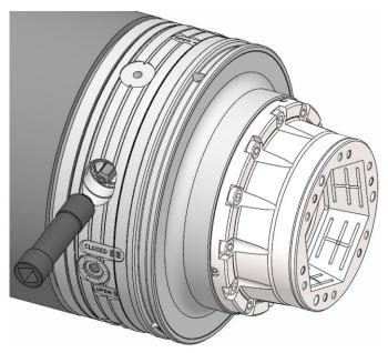
Remove the actuating key from the locking screw and remove it from the working area of the machine.
