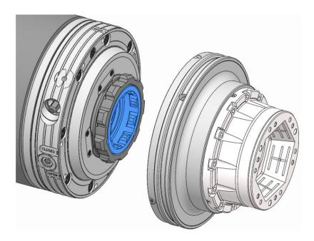
9. Fit the quick change-over unit to the machine adapter so that the mark on the quick change-over unit is aligned with the »OPEN« mark on the machine adapter.
