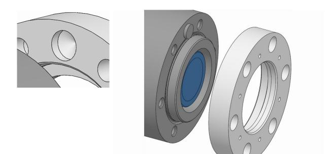
4. Take down the spindle flange from the machine spindle.
