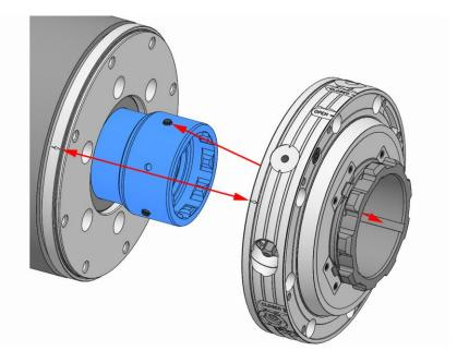
5. Fit the actuating unit on the spindle flange with the grooves in the actuating unit and the anti-twist device aligned with one another. For this, the marking on the spindle flange and the actuating unit must be aligned. For this, if necessary, twist the bayonet drawtube adapter.
