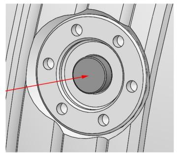
If the display pin protrudes after the locking screw has been tightened to the specified tightening torque, the quick change-over unit / quick change-over adapter has not been installed correctly. Use of the quick change-over system is prohibited if the quick change-over unit / the quick change-over adapter has not been installed correctly. The quick change-over unit / the quick change-over adapter must be installed again and the installation work must be inspected.
