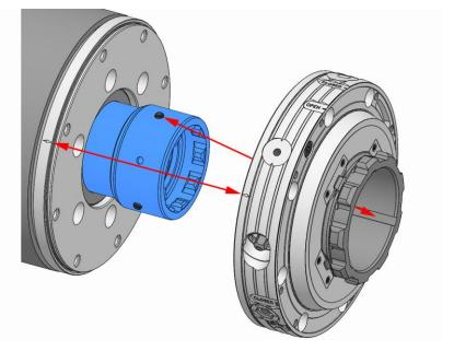
5. Remove the actuating unit from the spindle flange.
