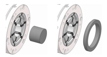
Install the dressing pin in the clamping device to prevent it from getting damaged when the HSW clamping head is getting machined. and/or, install the dressing ring firmly home in the turned groove in the HSW clamping head.
