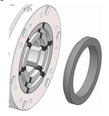
6. Remove the dressing pin from the clamping device. And/or remove the dressing ring from the HSW clamping head.
