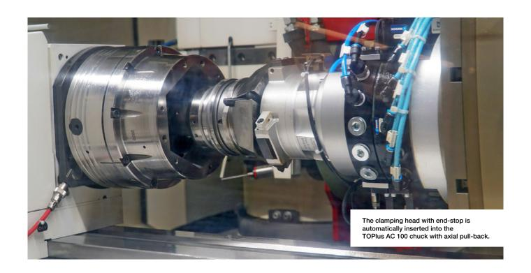
with axial pull-back. For the various housings, there are now 18 clamping sets, consisting of a clamping head with end-stop, which are automatically changed over in the chuck. However, for the I.D. clamping when turning and grinding, a completely new development was required. It was based on the existing MAXXOS T211 mandrel, however in this version with safety checks, a specific mandrel was developed.
