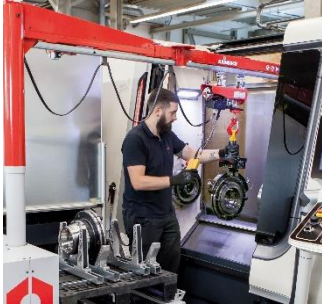
Photo: setup hoist-cantilever arm:
