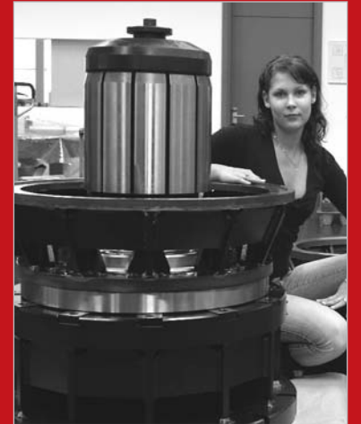
The largest HAINBUCH mandrel so far: Clamping range to 420 mm, weighing in at 1.3 tons.
