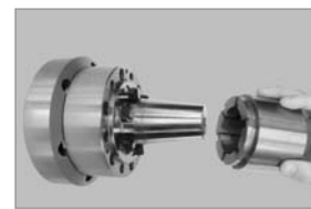
Pull off the segmented clamping bushing
