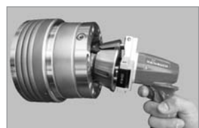
Take off clamping head
